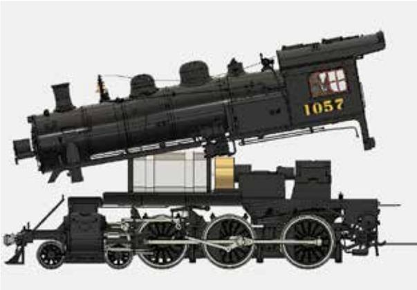
Tilting the boiler from the BACK forward (as depicted in the illustration) slide the boiler off. This will leave exposed the motor, universal, worm gear cover, and flywheel. Place the boiler in a safe place where not damage will occur.
