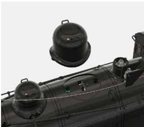
The smoke feature is controlled by a micro switch located underneath the sand dome. To remove the sand dome, you must pull **STRAIGHT** up. **DO NOT** lift on an angle. This will cause damage to the support pins.
