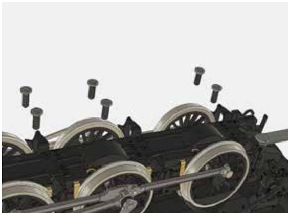
On the bottom of your locomotive, there are a series of 6 (six) screws that secure the gear cover on. Placing the locomotive on a secure work station, such as a foam cradle, remove these screws. Place these screws somewhere where you will not lose them. A small dish or container is suggested to hold these screws and stop them from rolling off your work station.
